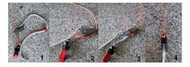
5. take the rope again through the bar and secure it to the quickrelease. Old Safety not need to be threaded again, it will be replaced in the next step.
