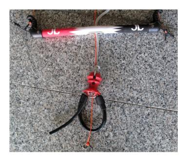
Are all the lines replaced or extended you should check if all lines are the same length.
