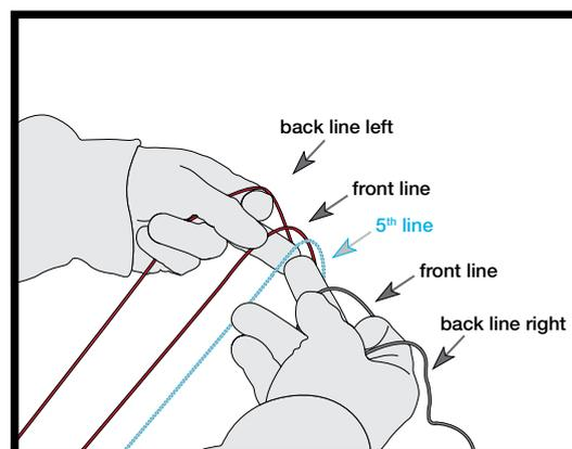
Connect your flying lines to the kite's pigtails by a simple larks head and ensure that they are set properly. Always check your set-up kite, ensuring untwisted lines twice before launching.
