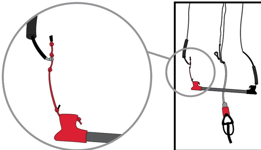
power" knot which extends the back- lines, so length difference gets balanced. Alternatively you can extend the backlines by moving the knots under the floats at the bar ends.
